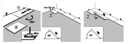
4) Fit the flooring tongue of the 2nd row into the groove of the 1st row, at an angle of 20-30°. Press it flat gently and fasten the flooring along the short side (board width) by using the striking block and hammer. This is to get the boards along the short side snug and tight. The rest of the installation should be installed in the same way.
